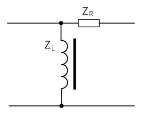
In line input applications you normally use high impedance transformers (transformers wound with many turns of thin wire), as the transformer inductive impedance  $Z_L$  is parallel to the following input circuit impedance.
